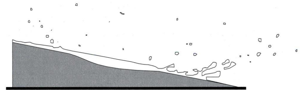
Fig. 15.7. Splash erosion on a sloping soil surface.
