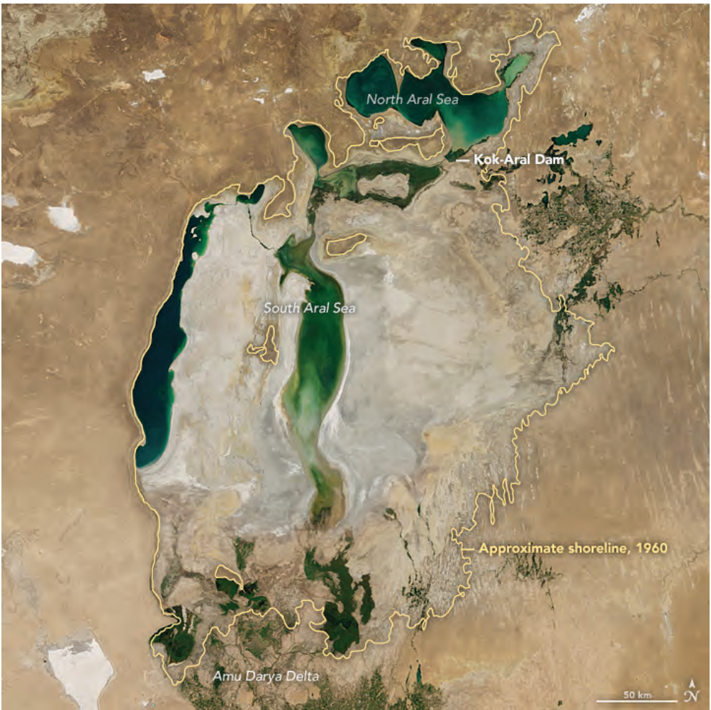
Satellite overview of the Kokaral dam. The positive effect of the dam is resulting in the expansion of the small Aral Sea. Source: NASA 4 .
